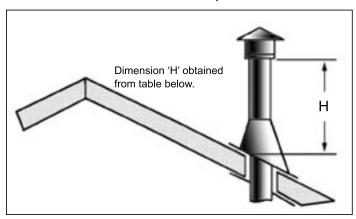
Figure 29: Height of Vertical Termination; Reference Table 6.
